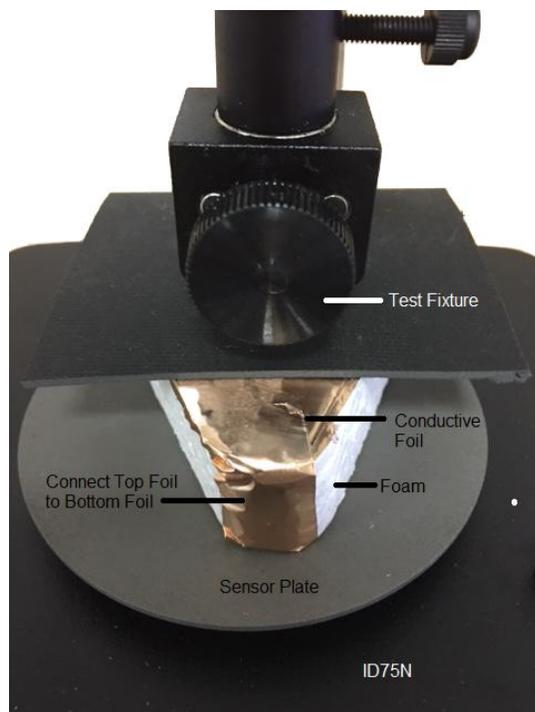
In the picture at left we have an example of a "Stepped Test" being conducted. The insertion layer is composed of 1lb. Styrofoam with a very thin layer of copper foil plating both top and bottom. When the small piece of conductive foil is adhered to both top and bottom plates a clear path of conductivity is established from the ID75N sensor plate to the puncture tool.
