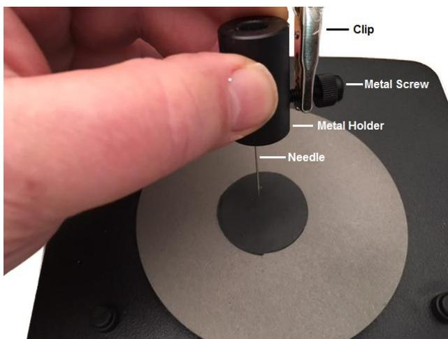
**Conductivity is maintained** because the clip is attached to the metal screw which is in secure contact with both the needle and the body of the metal holder. The body of the metal holder provides a safe and secure means of controlling the needle. If you do not require a mechanical fixture or holder then simply attach the clip directly to the needle and use the clip as a handle. You may need to "pinch" the jaws of the clip together to avoid slippage of the needle.
