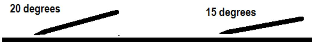
Generally speaking the 20° angle will be used for de-burring operations and the 15° angle will be used for edge straightening and periodic maintenance procedures. Remember...don't worry a lot about the preciseness of these angles because the SHARP PAD design has your back. If in doubt, error on the side of less angle and not more. Too much angle can reduce the sharpness of your edge.
